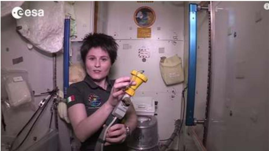
The astronauts urinate into a funnel that carries the liquid to where it is recycled into drinking water.
